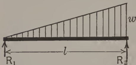
FIG. 103.—Non-uniformly distributed load.
